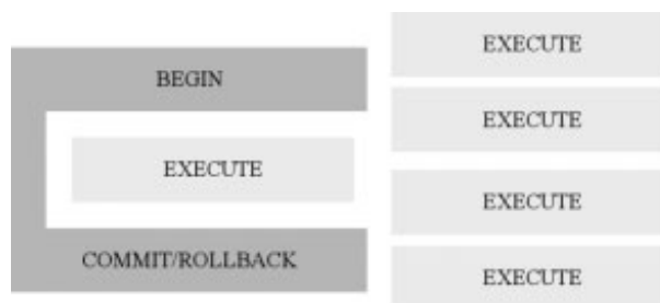
Figure 3 – A base class handles the BEGIN and COMMIT/ROLLBACK logic, with overridden EXECUTE methods containing data update logic. Data update methods are limited to a single class hierarchy
